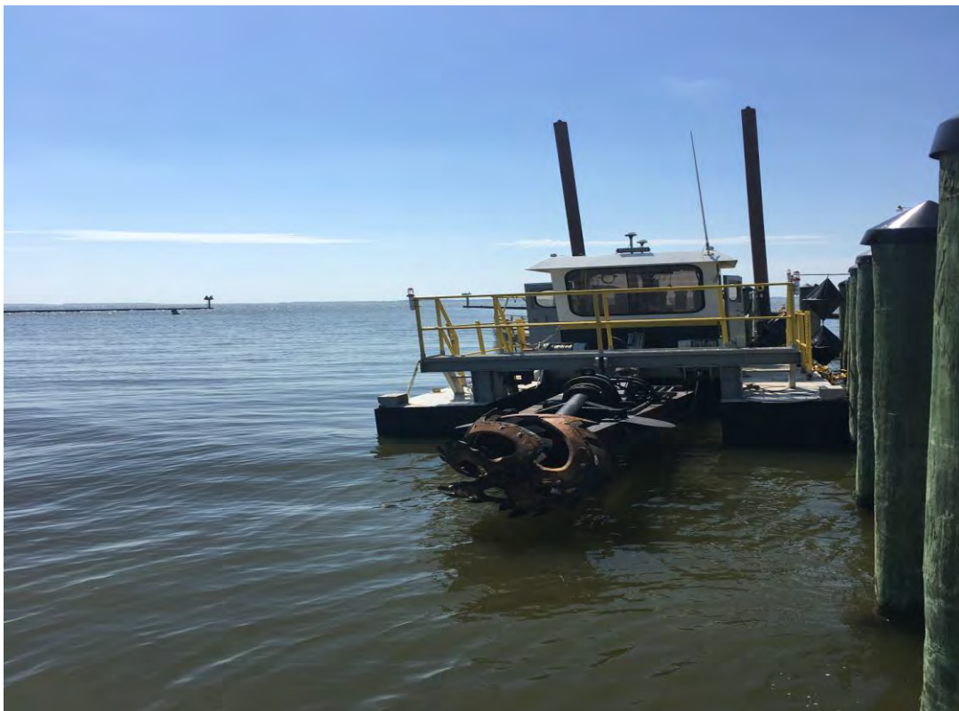
(Below) Photo 4: 2019 Hydraulic Dredge Plant, Chincoteague Inlet, VA. Source Credits: USACE and Dredgit Corp.
