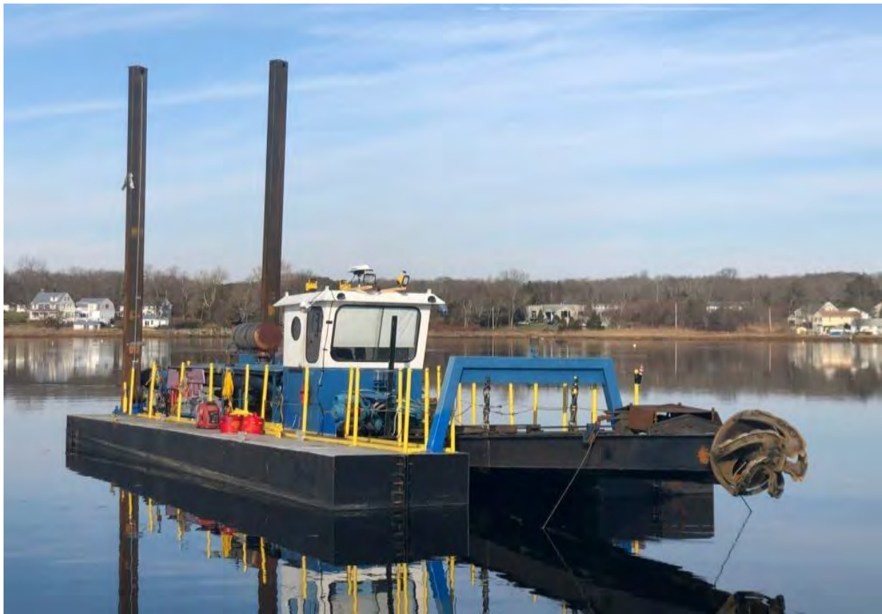
(Above) Photo 1: 2020 Hydraulic Dredge Plant, Oyster Channel, VA. Source Credits: USACE and Dredgit Corp.
